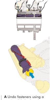
A Undo fasteners using a coin, slide back end caps and remove soleplate.
